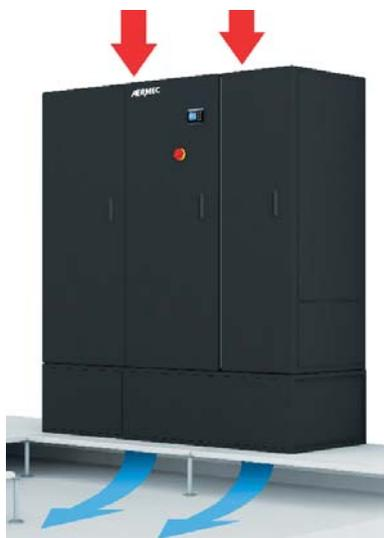
Standard version for data centre perimeter installation with raised floor height less than 550 mm. In this case the stand, having a fixed height of 550 mm provided with side closing panels, must be installed above the floor. However, please make sure that the ceiling height allows good air intake.
