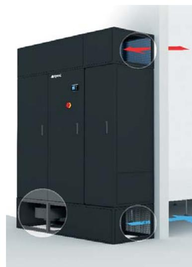
Version for installation outside the data centre, with no raised floor and rear supply line. In this case the stand, having a fixed height of 550 mm, is provided with side closing panels and rear supply grilles. The installation of a plenum with a rear air intake system is optional, in the absence of a duct system.
