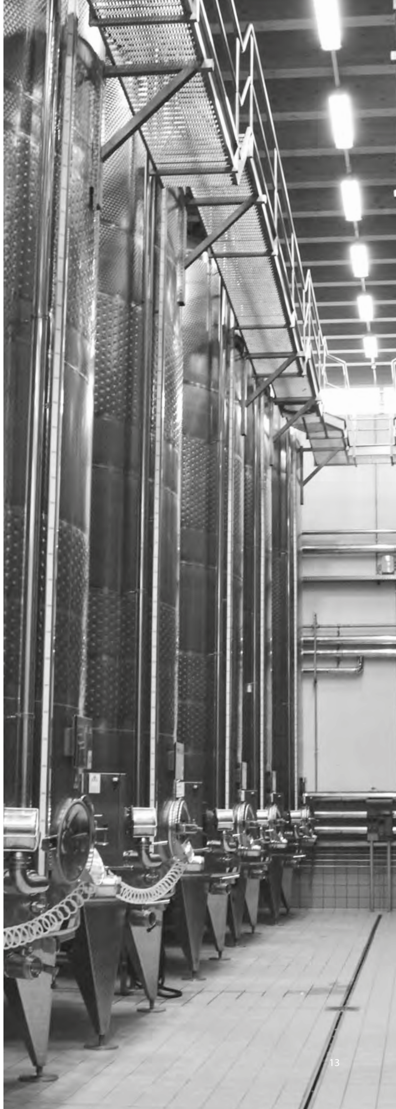
Cantina Vivallis. Tanks with thermal exchange jackets for temperature control
