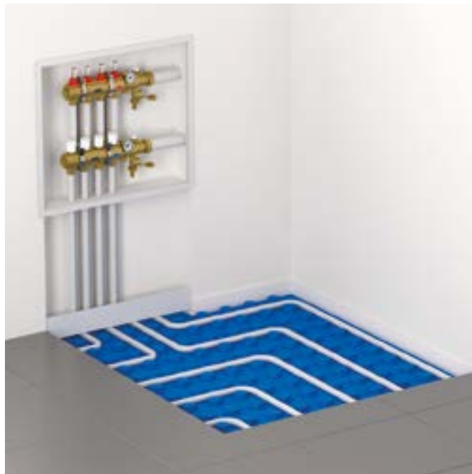
Radiant system made of multilayer pipe
